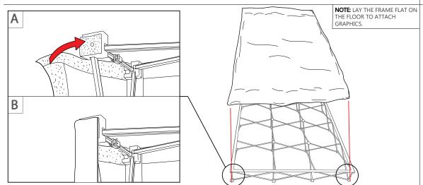
3 START AT A CORNER OF THE FRAME AND ATTACH THE GRAPHIC WRAP USING THE VELCRO. CONTINUE WORKING YOUR WAY AROUND THE FRAME WITH THE WRAP, INSURING A TIGHT FIT FROM CORNER TO CORNER.
