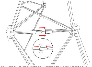
2 CONNECT ALL SIX OF THE RED CONNECTORS TO INSURE A SECURE AND STABLE CONNECTION.
