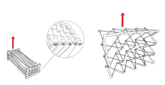
1 PLACE FRAME ON THE GROUND, INSURING THAT THE ORIENTATION HAS THE CIRCULAR FEET TOUCHING THE FLOOR. GRAB THE FRAME FROM THE CENTER AND LIFT UP TO EXPAND THE FRAME.
