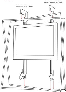
4. SECURE THE SYSTEM BY GENTLY PULLING THE UNIT DOWN ONTO ITS CORRESPONDING POINTS ALONG THE FRAME.
