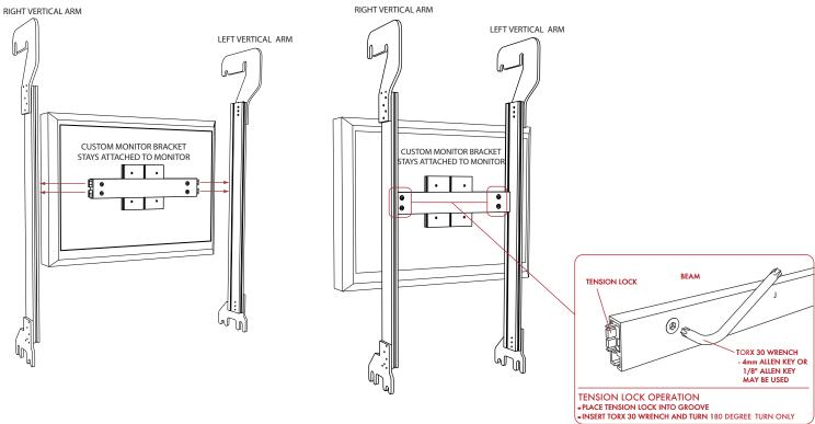
3. LINE THE MONITOR'S CENTER WITH THE CENTER PIVOT OF THE FRAME. THEN GENTLY HOOK THE UNIT OVER THE TOP BARS.
