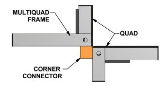
AFTER TWO MULTIQUAD FRAMES ARE SET "CORNER-TO-CORNER" THE MQ-BTW SIMPLY ATTACHES TO THE EXISTING MAGNETS ON THE FRAME
